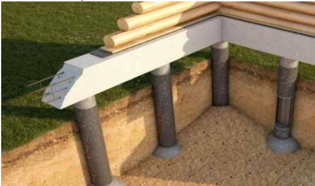
Fig.1: Pile Foundation Construction
